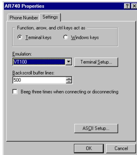
6 Click “ASCII Setup” to display the ASCII Setup dialog box. Uncheck the “Echo typed characters locally” and “Append line feeds to incoming line ends” checkboxes. Set other parameters as required, then click “OK” twice to dismiss all dialog boxes.
